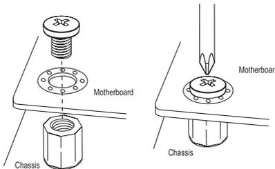
6. Using the Phillips screwdriver, insert a Phillips head #6 screw into a mounting hole on the motherboard and its matching mounting hole on the chassis.
