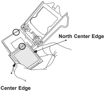
4. Align the CPU key that is the semi-circle cutouts against the socket keys. Once it is aligned, carefully lower the CPU straight down into the socket. (Do not drop the CPU on the socket. Do not move the CPU horizontally or vertically.)
