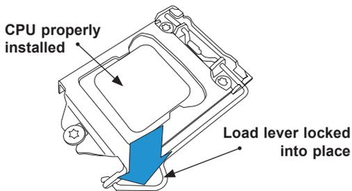
**! Attention!** You can only install the CPU inside the socket only in one direction. Make sure that it is properly inserted into the CPU socket before closing the load plate. If it doesn't close properly, do not force it as it may damage your CPU. Instead, open the load plate again and double-check that the CPU is aligned properly.
