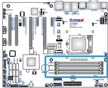
2. Push the release tabs outwards on both ends of the DIMM slot to unlock it.
