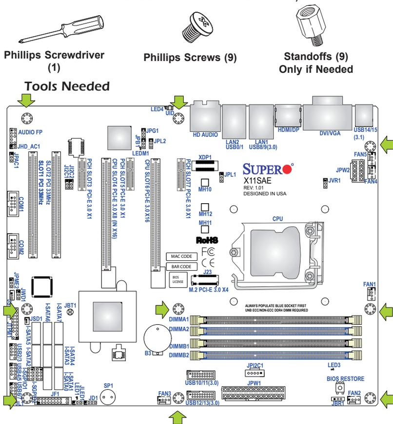
**! Attention!** 1) To avoid damaging the motherboard and its components, please do not use a force greater than 8 lb/inch on each mounting screw during motherboard installation. 2) Some components are very close to the mounting holes. Please take precautionary measures to avoid damaging these components when installing the motherboard to the chassis.
