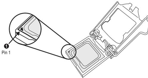
6. With the CPU inside the socket, inspect the four corners of the CPU to make sure that the CPU is properly installed.
